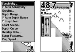
Sonar Menu with Sensitivity command selected (left). Sensitivity Control Bar (right).
